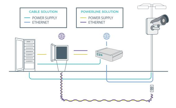
Park smart system could be installed next to camera or, with and additional kit based on powerline, close to the electrical panel that supply cameras. The unique qualities of Park Smart are:
